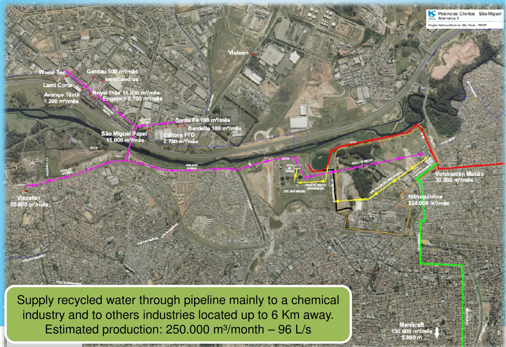
Supply recycled water through pipeline mainly to a chemical industry and to others industries located up to 6 Km away.
