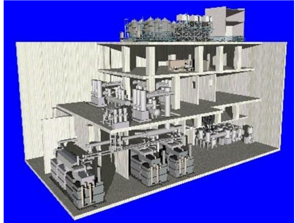
Layout of Underground Substation
